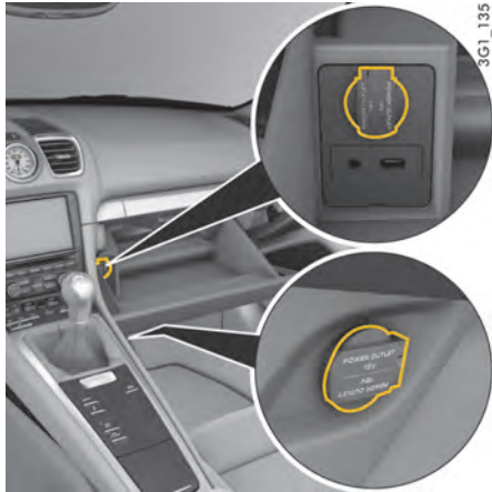
Sockets in the glove box and passenger footwell
